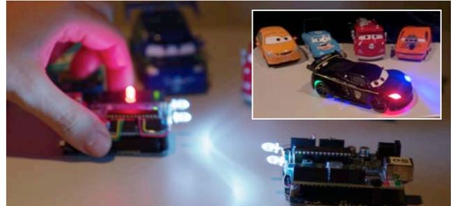
**Figure 1.** Toy car scenario (Mangold 2012). Networked toys equipped with LEDs exchange messages. A communication distance of up to one meter at one kilobit per second is demonstrated.
